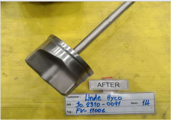
The metal touch surface of seat ring was good after clean and lapping.
