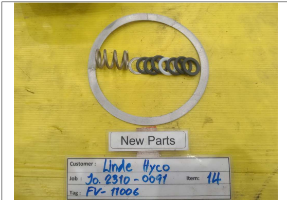
The new soft parts of body were inspected before replacement on this maintenance period.
