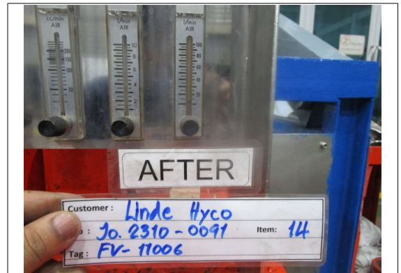
This valve has a seat leakage tested and executed a body pressure test, the result of tested was good.
